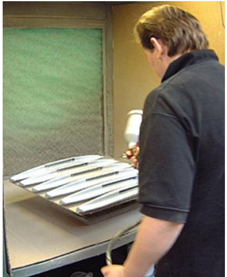
Appliance handles being sprayed with Indestructible's PBT coating system.
