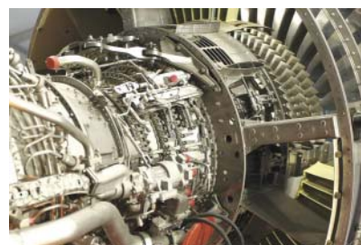
1 A gas turbine engine. The various coatings used on internal and external engine components need to provide protection against one or more of the following: an extremely corrosive environment, very high temperature, erosion and chemical attack
