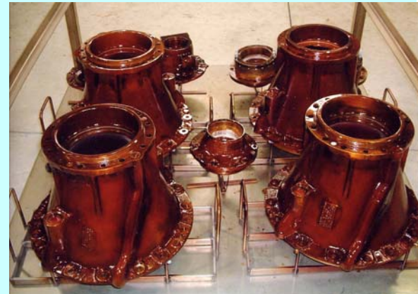
Magnesium helicopter gearbox casings coated in Rockhard
